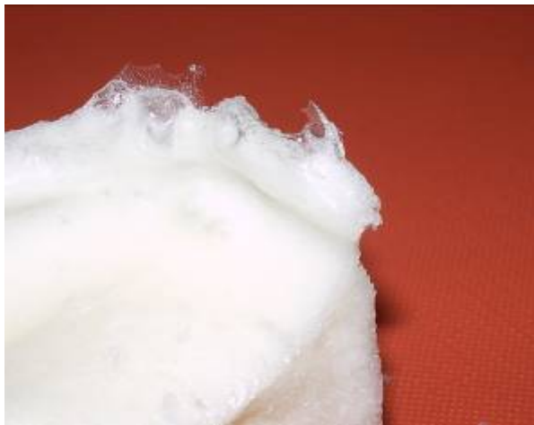
Pic.2 MEYCO ® MP 350 foamed after reaction with water excess
